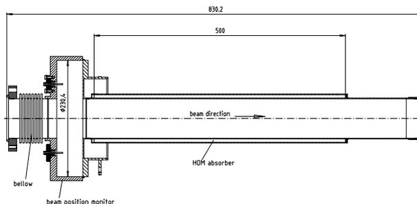
Figure 1: Cold cavity BPM with HOM absorber
