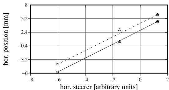
Figure 7: Beam deflection vs. steering - Full line (circles) = stripline readout; dashed line (triangles) = image center.
