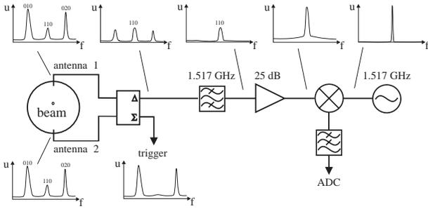
Figure 2: Signal processing scheme for a cavity BPM
