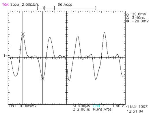
Figure 5: Measured signal for a stripline BPM
