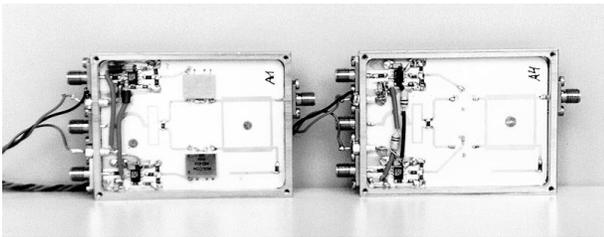
Figure 3: Realized I/Q-mixers: MD-164 (left) and M2G
