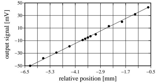
Figure 4: Test at CTF - output versus rel. position
